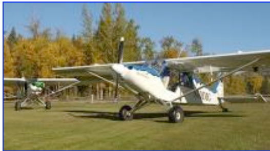
The Mountain Goat, foreground, can carry more cargo over a longer distance, has a slower stall speed and cruises faster than the Super Cub. (Photo by Bill Roth / Anchorage Daily News)
